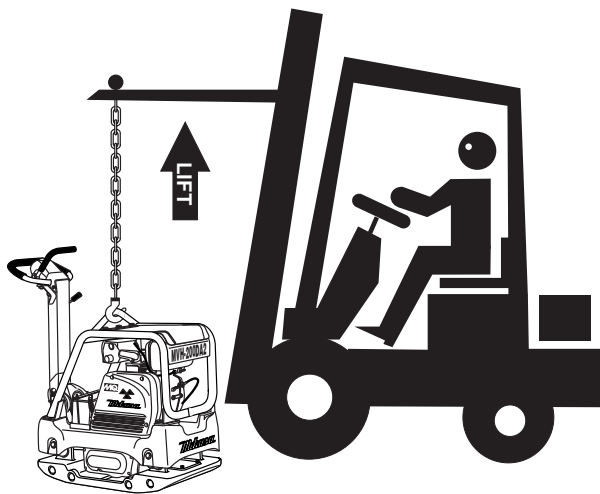
Figure 18. Lifting the Compactor
