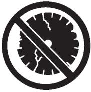
Failure to thoroughly inspect the blade for operational safety could result in damage to the blades or the saw and may cause serious injury to the user or others in the operating area. Inspect the blade flanges and shaft for damage before installing the blade.
