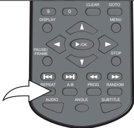
While in the Playback mode, press the REPEAT button once; “ TRACK” will appear on the screen and the currently playing track will repeat continuously.
