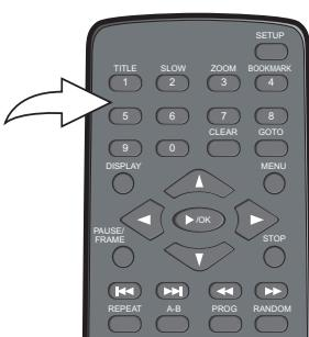
During playback, press the Number buttons corresponding to the track number to select your desired track, and the unit will playback the desired track automatically.
