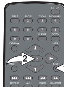
Close the disc tray. After loading, the menu screen of the DVD should appear. Use the Navigation ( $\blacktriangleleft$ ,  $\blacktriangleright$ ,  $\blacktriangleup$ ,  $\blacktriangledown$ ) buttons ① to select the desired option and press the PLAY ( $\blacktriangleright$ )/OK button ② to select it. Adjust the VOLUME control ③ as desired.
