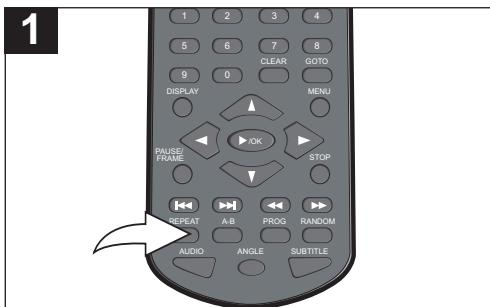
While in the Playback mode, press the REPEAT button once; “ CHAPTER” will appear on the screen for a few seconds and the currently playing Chapter will repeat continuously.
