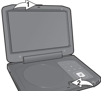
Slide the POWER ON/OFF switch to the ON position to turn the unit on; the POWER indicator will light. (Make sure that the AV IN/OUT switch is in the OUT position. Otherwise, the display will not show a picture.)
