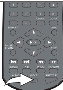
Press the ANGLE button repeatedly to select an alternate angle.
