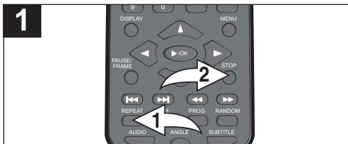
Press the REPEAT button ① to cycle through the following options: SINGLE (will playback the selected file once and then stop), REPEAT ONE (will repeat the selected file continuously until the STOP button ② is pressed), REPEAT FOLDER (will repeat the selected folder continuously until the STOP button ② is pressed) or FOLDER (will playback the selected folder once and then stop).
