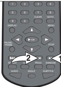
During playback, press either the Search ►► button ① or Search◀◀ button ② to move the DVD forward or backward at double (x2) speed to locate a specific section. Repeatedly press these buttons and the speed will increase to x4, x8, x16, x32 and resume normal playback.
