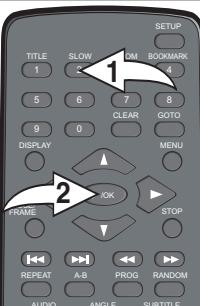
During playback, press the SLOW button ① to move the DVD forward in slow motion speeds of 1/2, 1/4, 1/8, 1/16 and resume normal playback. The sound will be muted. You can also resume normal playback by pressing the PLAY (▶)/OK button ②.
