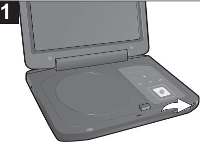
1 Slide the POWER ON/OFF switch to the ON position to turn the unit on; the POWER indicator will light.
