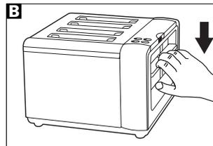
Use the front bread lever to activate the high lift function for the two and four slices.
