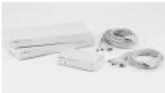
**Console Switch** – A device that allows a user to operate multiple servers with a single keyboard, monitor, and mouse.
