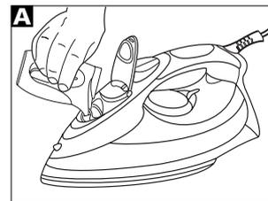
After filling, replace the fill cap. In hard water areas, the use of distilled or demineralised water is recommended.
