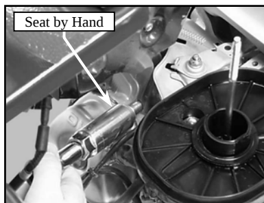
(E) Install the Spark Plug by Hand DO NOT cross-thread the Spark Plug
