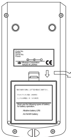
Push down the stopper of the battery box and pull forward.
