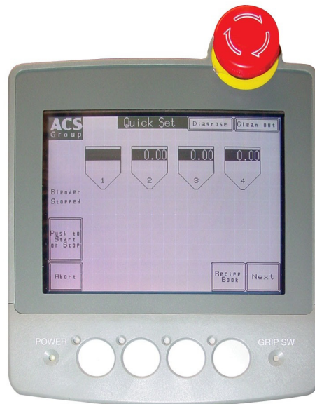
Figure 4: Typical Mitsubishi Controller Touch Screen Display
