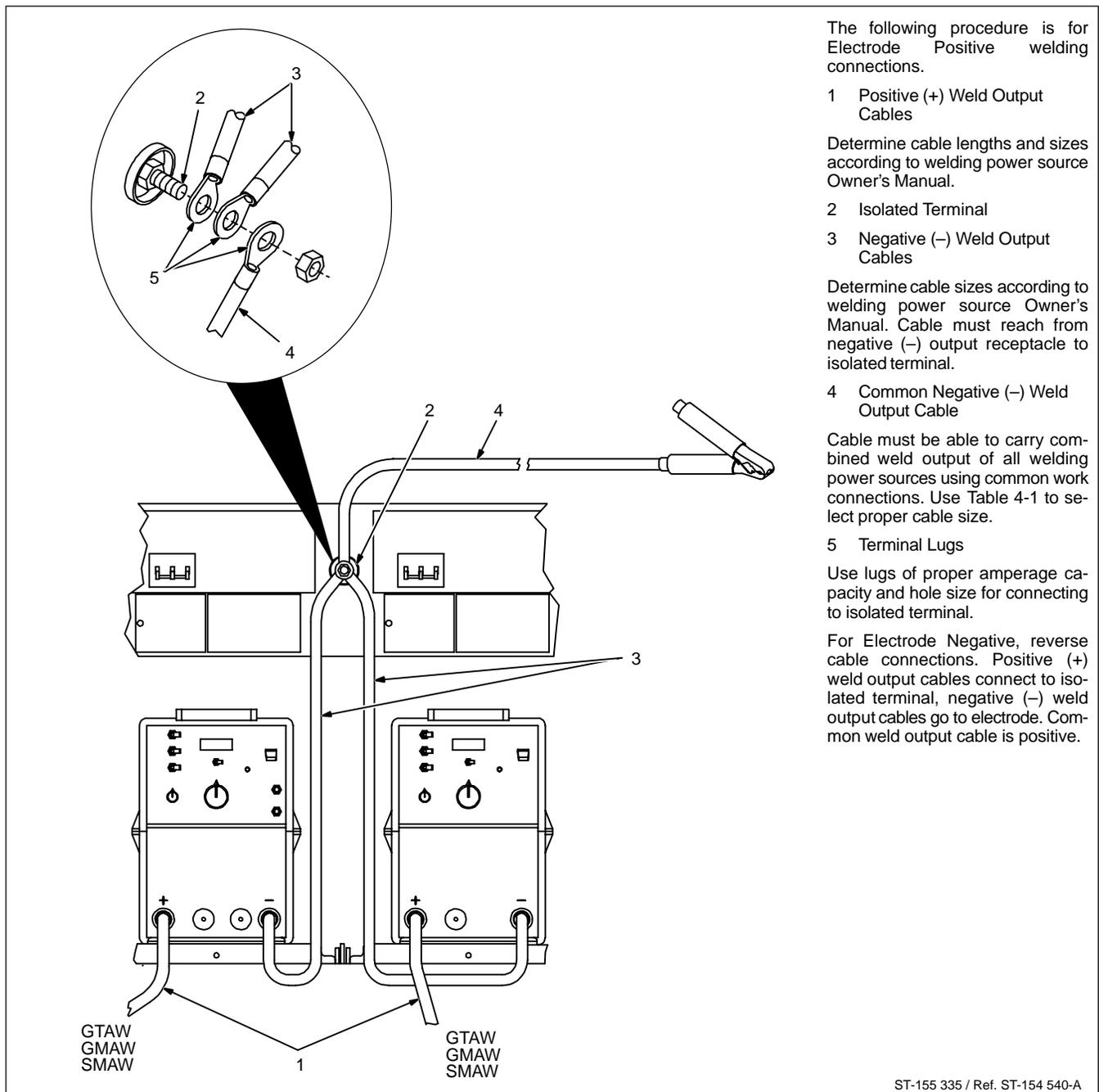
Figure 4-4. Common Work Connections
