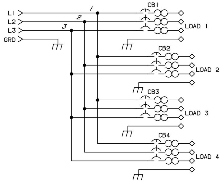
Figure 6-1. Circuit Diagram For Rack Control Box
