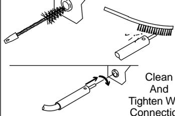
Clean And Tighten Weld Connections
