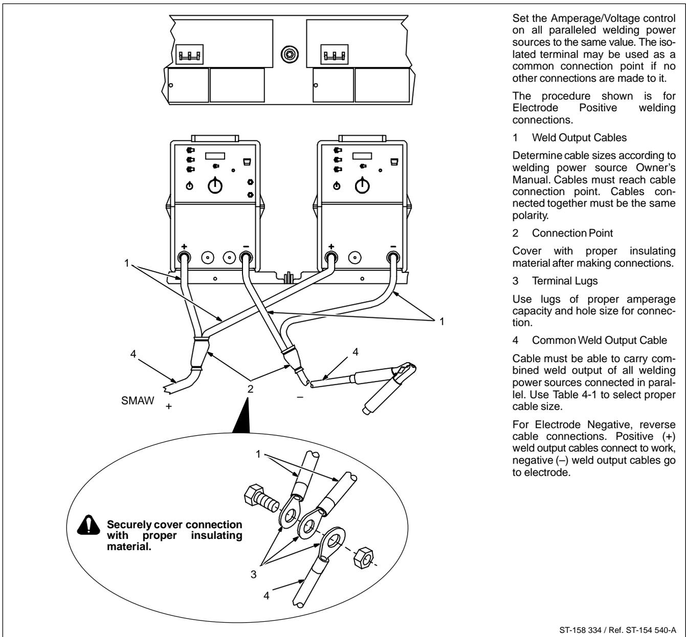
Figure 4-5. Paralleling Welding Power Sources For SMAW
