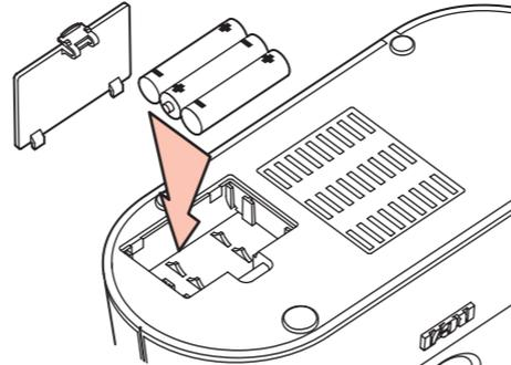
Follow the polarity markers in the battery compartment.
