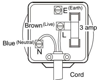
The wire coloured BLUE must be connected to the terminal marked N or coloured BLACK.
