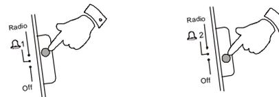
2. Press the **Alarm Set button** to display the alarm 1 time.
