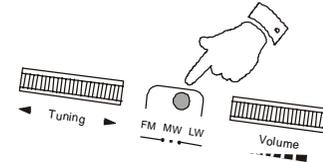
3. Tune in to the desired station by rotating the **Tuning control**. The station frequency is indicated by the **LED dial pointer**.
