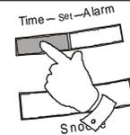
4. Whilst holding down the **Time Set** button press the fast forward (**F-Fwd**), slow forward (**S-Fwd**) or slow reverse (**S-Rev**) buttons to set the time. Release the buttons when the correct time is reached. The clock uses a 12 hour display with a **PM indicator**. Ensure that the correct 12 hour cycle is selected.
