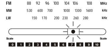
2. Select the required waveband using the **Waveband selector switch**.
