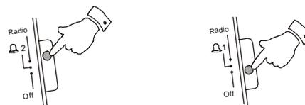
4. Press the **Alarm Set button** to display the alarm 2 time.
