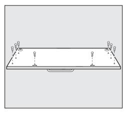
⑦ Screw the removed panel to the custom panel with the eight screws.
