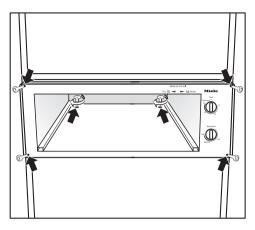
• Secure the casing in the cabinetry with the six screws.
