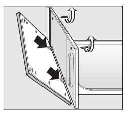
(a) Hook the panels into the bottom on and secure at the top with two screws making sure the seal is seated correctly. When contacting the Technical Service, please quote the model and serial number of your appliance.
