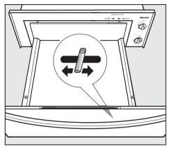
The humidity control adjusts the humidity within the drawer. The humidity control can be set anywhere between "Moist" and "Dry".
