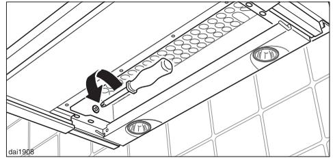
Note for dismantling the cooker hood: Undoing the screws on the left and right inside the housing releases the brackets, allowing the appliance to be removed from the unit.
