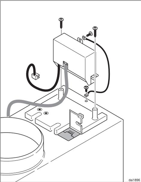
The control module must be installed above the cooker hood housing.
