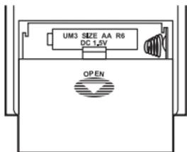
2. Place the batteries in the compartment as indicated by the polarity symbols (+ and -) marked inside.
