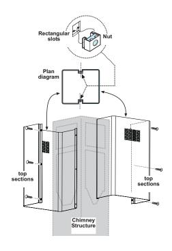
**13.** Install top duct covers assembly to the chimney structure.
