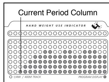
Current Period column of the program display. (The incline settings are not shown in the program display.) The speed settings for the next seventeen periods are shown in the seventeen columns to the right.
