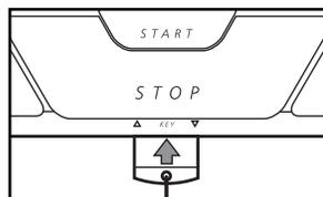
Next, insert the key into the console. After a moment, the displays, the LED track, and various indicators on the console will light.
