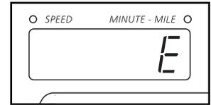
**Time/Segment Time display**—When the manual mode or an iFIT.com program is selected, this display will show the elapsed time. When a performance program, a total-body workout program, or a custom program is selected, the display will show both the time remaining in the program and the time remaining in the current period of the program. The display will alternate between one number and the other every seven seconds.
