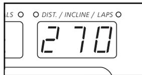
An "E" for English miles, or an "M" for metric kilometers, will appear in the Speed/Minutes-Mile display. Press the Speed  $\Delta$  button to change the unit of measurement.
