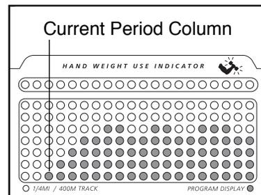
When only three seconds remain in the first period of the program, both the Current Period column and the column to the right will flash, a series of
