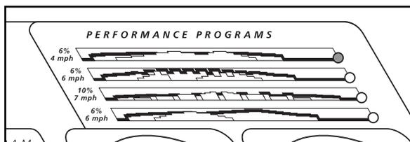
The profiles on the console show how the speed and incline of the treadmill will change during the programs. The numbers at the left ends of the profiles show the maximum speed and incline settings for the programs. For example, the profile for the first performance program shows that the treadmill will reach a maximum incline level of 6% and a maximum speed of 4 mph during the program.
