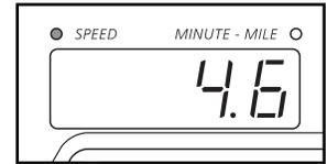
Note: The console can display speed in either miles per hour (mph) or kilometers per hour (kph). To see which unit of measurement is selected, first hold down the Stop button while inserting the key into the console. The Speed/Minutes-Mile display will show an “E” for English miles or an “M” for metric kilometers. Press the Speed  $\Delta$  button to change the unit of measurement. When the desired unit of measurement is selected, remove and then reinsert the key.
