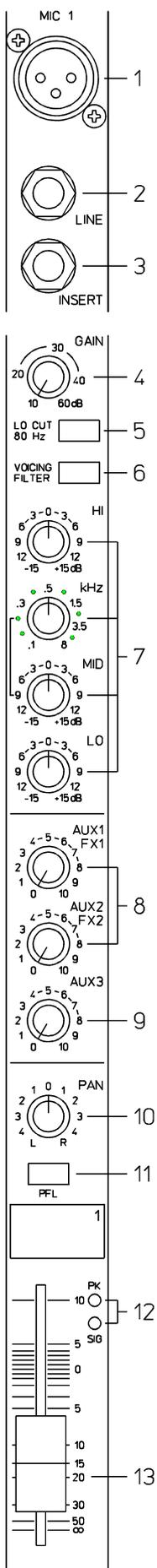
If you want to use this socket as a DIRECT OUT (Pre EQ), the stereo phone plug's tip and ring have to be short circuited, so that the audio signal is not interrupted. If you are using a monaural phone plug instead, you will get a DIRECT OUT with breaker function – the signal flow within the channel is interrupted.
