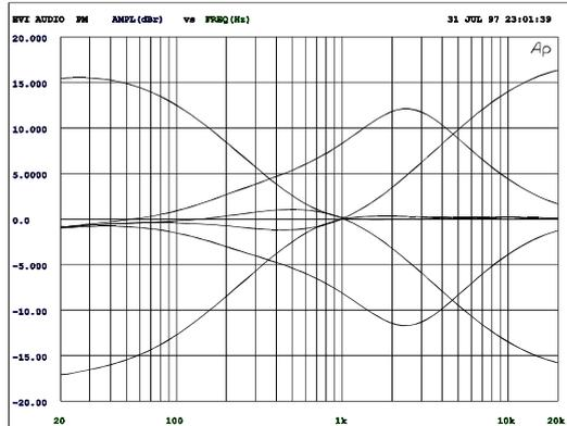
The HI and LO controls of the STEREO channels' EQ section provide a degree of control that is equally adequate for LINE level inputs and microphones. The MID control is active in a comparably wide frequency band around 2.4 kHz. With most microphones this is the critical range, where a slight attenuation offers excellent results.
