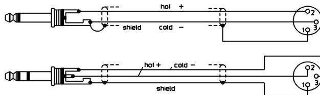
**unbalanced** external equipment with XLR-type in/output jacks
