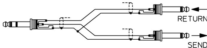
Y-type cable for the connection of external FX units and signal processors with phone jacks
