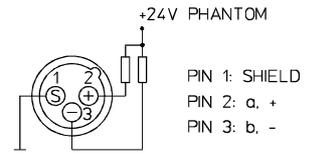
**CAUTION:** Make sure to always connect the microphones before turning on the phantom power or switching the PSX on with phantom power activated. This is the only way to prevent your microphones from damage. Also be sure to engage the stand-by button in the master section to prevent nasty power-on transients.
