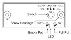
the sensor while calibrating because this will cause a false reading. Using a small nonmetallic screwdriver or alignment tool, turn trimpot Full until the LED just lights, and no farther. Note the position. Now turn the trimpot back until the LED turns off. The ideal setting for the trimpot is midway between these on and off points.
