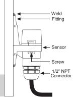
If desired, the sensor may be installed temporarily without welding the fitting to the wall. If several different locations must be tried before permanent installation, use double-sided foam stick tape designed for PE, for example Arclad type PE-6024, CO#7331 (from Adhesive Research Inc., Glen Rock PA 17327) or equivalent.
