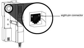
The RJ-45 connector is an eight-pin female connector. The eight pins connect horizontally along the top. Pin 8 has the leftmost position, and pin 1 is the rightmost. The pin-out for the RJ-45 complies with the information in the following table:
