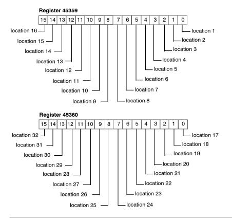
**Node Assembly** The next eight contiguous registers (registers 45367 through 45374) indicate the presence or absence of configured modules in locations on the island bus. This information is stored in Flash memory. At start up, the actual locations of the modules on the island are validated by comparing them to the configured locations stored in memory. Each bit represents a module:
