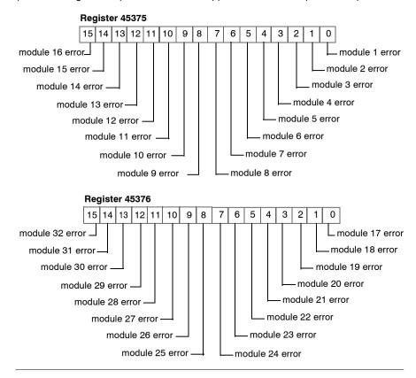
**Fault Detection** The next eight contiguous registers (registers 45383 through 45390) indicate the presence or absence of operational faults detected on the island bus modules. Each bit represents a module:
