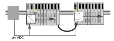
The logic power signal is terminated in the STB XBE 1000 module at the end of the segment (EOS).
