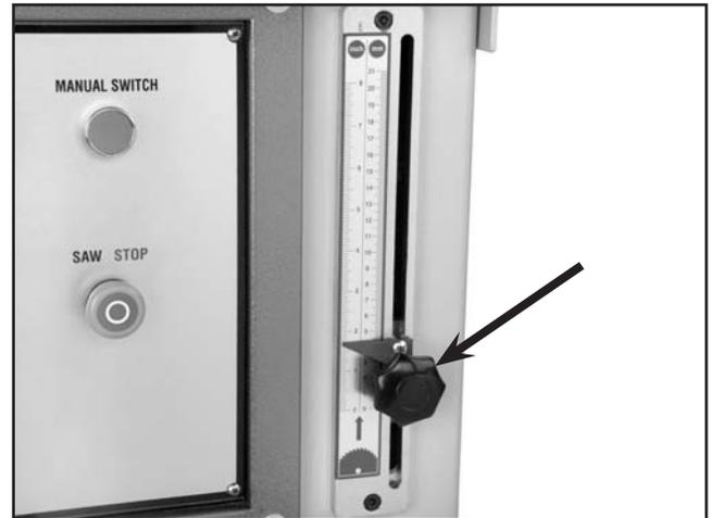
**Figure 35. Blade stroke height lock knob.**
