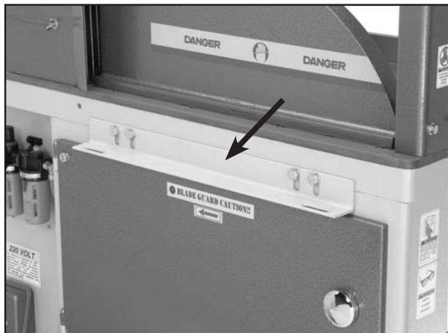
**Figure 9.** Mounting bracket attached to saw.
