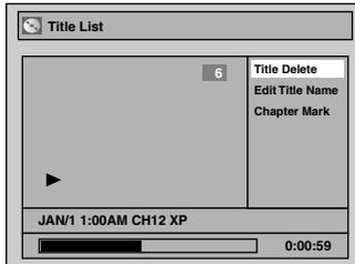
You cannot select “Chapter Mark” when a DVD-R disc is inserted into the unit.
