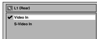
5. Using [▲ / ▼], select the input jack type to connect. Hit [ENTER].
