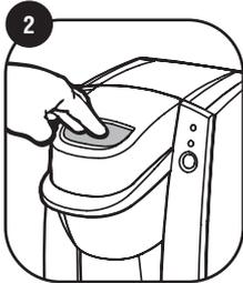
2 Depress the large "PRESS TO OPEN" button on top of the brewer.
