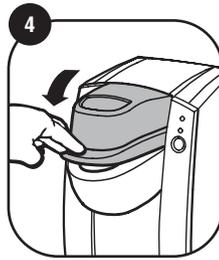
4 Lower the Handle completely and firmly to close the Lid and puncture the K-Cup® portion pack.
