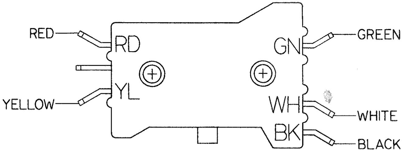
The above procedure can be used on all one speed washers except for the 132 and 132S. Below is the wire harness hookup for the 132 and 132S.
