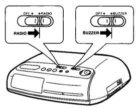
The radio alarm and the buzzer alarm are set at the same time, both alarms will activate simultaneously.
