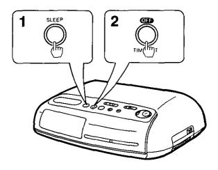
You can set the clock radio to play up to 59 minutes, then shut off automatically.
