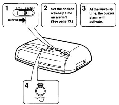
1 Set the alarm 2 selector to "BUZZER".
