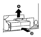
1 Connect a 9-Volt battery (not included) to the snaps, observing correct polarity.
