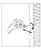
Loosen hex nut on door latch. Turn hook clockwise to tighten as shown. Secure hex nut firmly against door latch.
