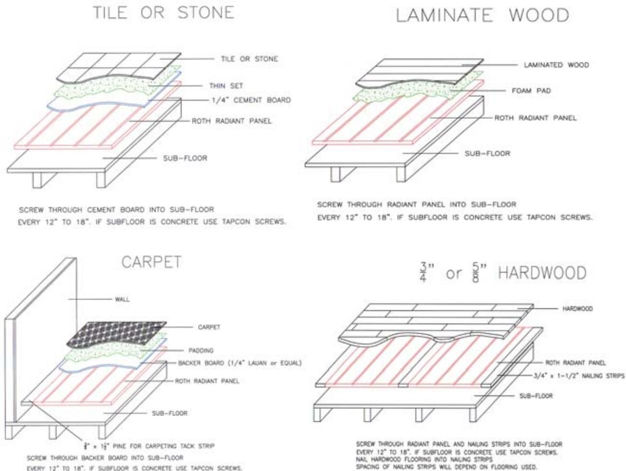
**Tile/Stone:** Roth recommends using a tile underlayment product in all ceramic tile installations. Underlayment should be secured and seams finished per manufacturer's instructions. It is also a good idea to use plasticizer additives with the mastic and grout for more flexibility during operation of the heating system.
