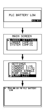
When a conveying problem occurs, the screen displays the alarm message and the audible alarm sounds.
