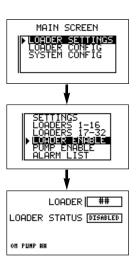
To enable the pumps from the main screen:
