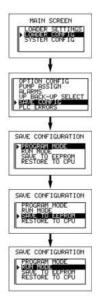
To back up the PLC program and save the configuration:
