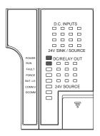
The controller status LEDs provide a mechanism to determine the current status of the controller if a programming device is not present or available.
