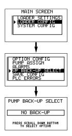
A backup pump can be assigned to replace any of the eight pump systems during operation.
