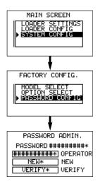
The B32 provides password security to prevent unauthorized changes to loader or system settings.
