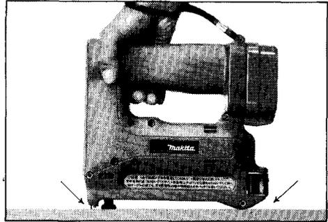
If the staples are driven too shallow, press the tool head as shown in the figure and drive the staples.
