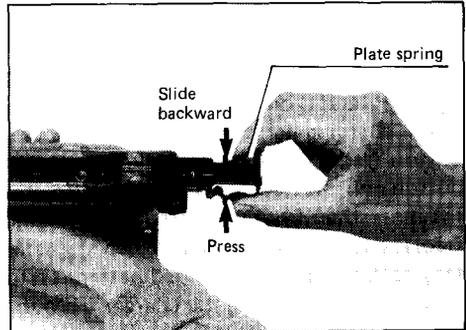
Load staples into the main magazine with staple ends facing up as illustrated at right. Slide the sub-magazine forward.
