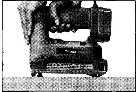
If the tool becomes jammed, do as follows. First, remove the battery cartridge. Open the sub-magazine and remove the stuck staple using a screwdriver or the like.
