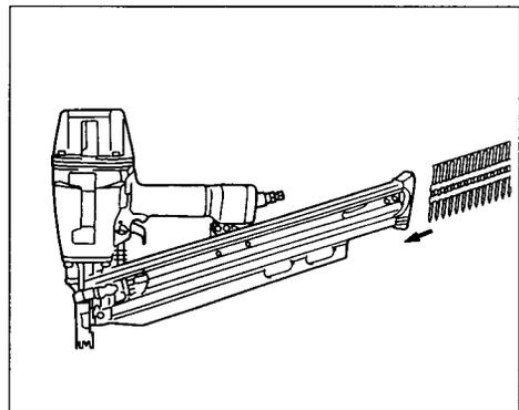
Pull the pusher lever to the rear to engage the pusher to the last nail.
