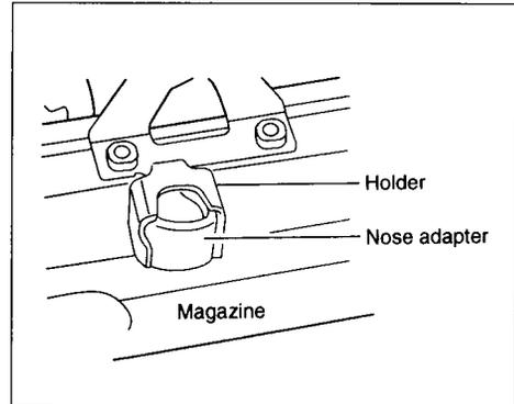
Attach the nose adapter to the contact arm (see right). When not in use, store the nose adapter in the holder on the reverse side of the magazine to keep it from being lost.
