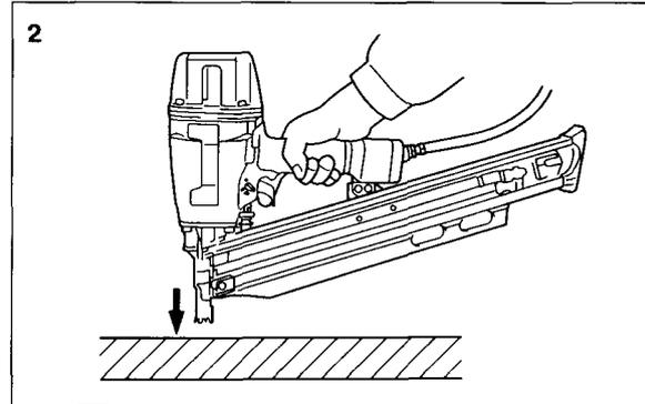
For No. 1 method, set the change lever to the "Intermittent Nailing" position.
