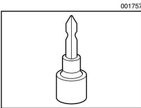
Hold the tool firmly with both hands whenever possible and place the socket over the bolt or nut. Then turn the tool on. As soon as the bolt or nut becomes tight, the clutch will cut in and the motor will stop automatically. Release the switch trigger.
