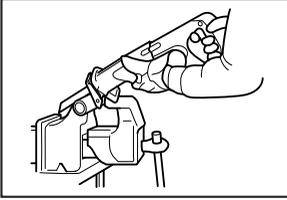
Press the shoe firmly against the workpiece. Do not allow the tool to bounce. Bring the blade into light contact with the workpiece. First, make a pilot groove using a slower speed. Then use a faster speed to continue cutting.
