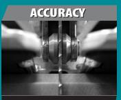
Blade roller guide is positioned close to the workpiece to guarantee accurate straight and bevel cuts
