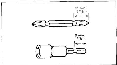
To install the bit, pull the sleeve in the direction of the arrow and insert the bit into the sleeve as far as it will go. Then release the sleeve to secure the bit.
