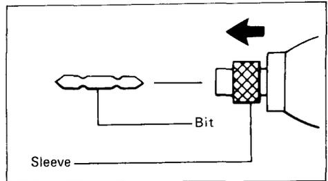
To remove the bit, pull the sleeve in the direction of the arrow and pull the bit out firmly.
