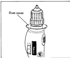
To remove the dust cover, slide it off firmly while turning it back and forth.
