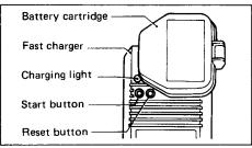
If the charging light does not come on, press the reset button (yellow) first, then the start button (red). If the charging light goes out within 10 seconds even after pressing the reset button and start button a couple of times, the battery cartridge is dead. (CAUTION: Wait for more than 5 seconds after the charging light goes out to press the reset button again.) Replace it with a new one. When the charging light goes out after about one our, you may remove the fully charged battery cartridge.
