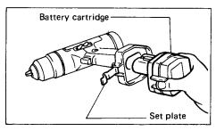
Do not use force when inserting the battery cartridge.
