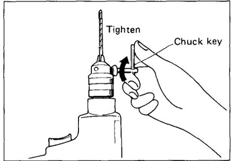
After using the chuck key, be sure to return it to the original position.
