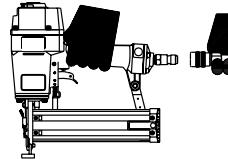
5. Depress the Work Contact Element (WCE) against the work surface without pulling the trigger. The nailer **MUST NOT OPERATE**. Do not use the tool if it operates without pulling the trigger. Personal injury may result.
