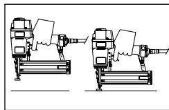
The trigger must be released to reset the tool before another nail can be driven.
