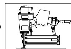
6. Remove the nailer from the work surface. The Work Contact Element (WCE) must return to its original down position. The nailer **MUST NOT OPERATE**. Do not use the tool if it operates while lifted from the work surface. Personal injury may result.
