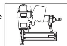
7. Pull the trigger and depress the work contact element (WCE) against the work surface. The nailer **MUST NOT OPERATE**.
