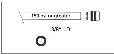
4. Use a pressure regulator on the compressor, with an operating pressure of 0 - 125 psi. A pressure regulator is required to control the operating pressure of the nailer between 70 and 110 psi.
