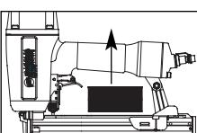
3. Make sure the trigger and work contact element (WCE) move freely up and down without sticking or binding.
