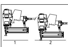
8. Depress the Work Contact Element (WCE) against the work surface. Pull the trigger. The nailer **MUST OPERATE**.
