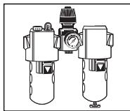
3. Always use air supply hoses with a minimum working pressure rating equal to or greater than the pressure from the power source if a regulator fails, or 150 psi, whichever is greater. Use 3/8" air hose for runs up to 50'. Use 1/2" air hoses for 50' run or longer. For better performance, install a 3/8" quick plug (1/4" NPT threads) with an inside diameter of .315" (8mm) on the nailer and a 3/8" quick coupler on the air hose.
