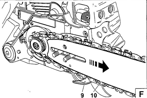
Line up the holes in the sprocket guard (3) with the bolts (11).
