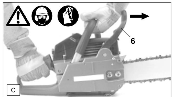
**Do not work with the chain saw without first checking the chain brake!**
