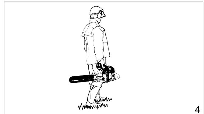
**By hand:** When carrying your saw by hand, the engine must be stopped and the saw must be in the proper position. The chain protection cover should be over the chain and the guide bar must point backwards. When carrying your saw the bar should be behind you (fig. 4).
