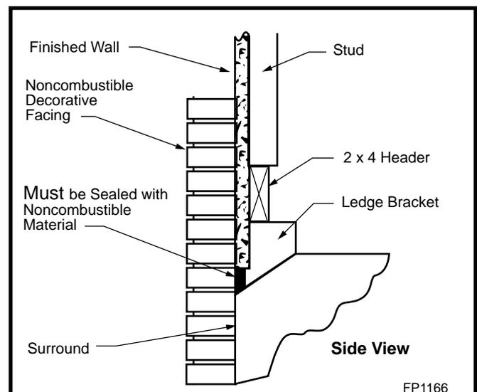
Fig. 19 Fireplace surround flush with finished wall.
