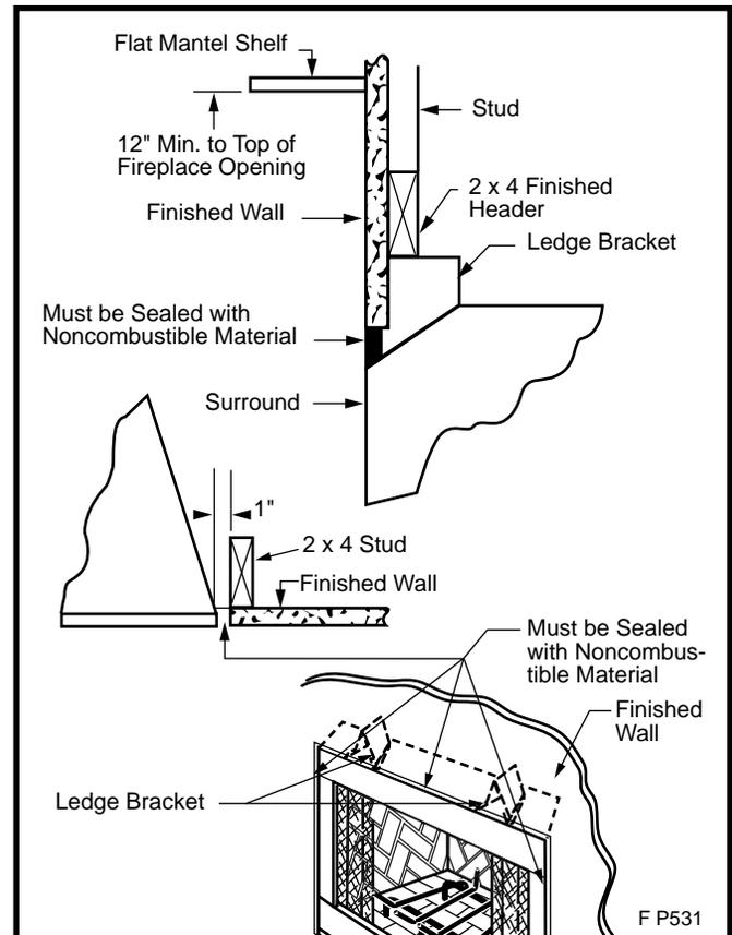
Fig. 18 Fireplace surround flush with finished wall.
