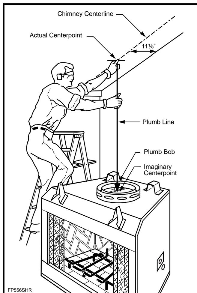
Fig. 9 Locate centerline of chimney with plumb line.
