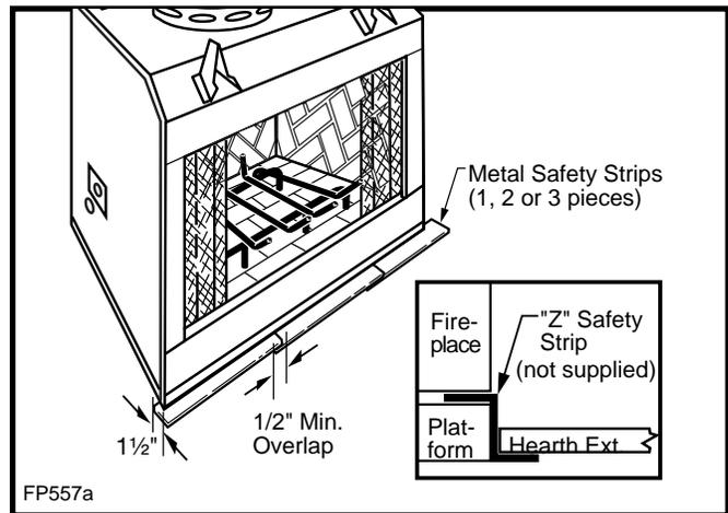
Fig. 12 Safety strip installation.
