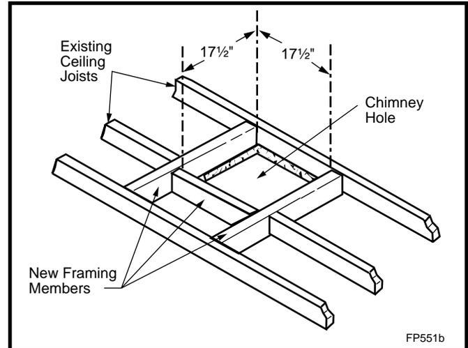
**Fig. 11** Typical frame for ceiling chimney hole.
