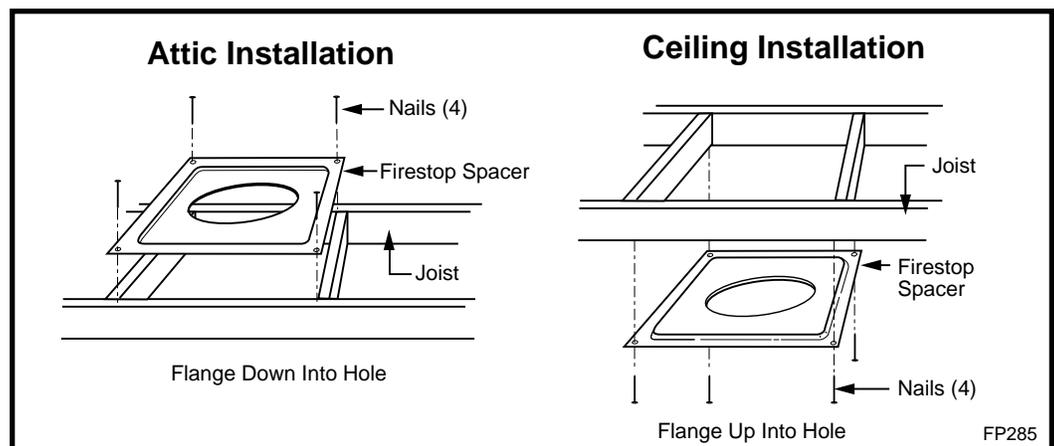
Fig. 16 Installing firestop spacer.
