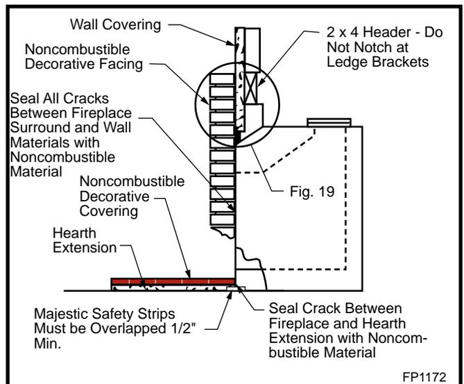
Fig. 28 Sealing detail.
