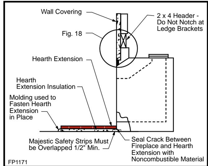
Fig. 27 Sealing detail.
