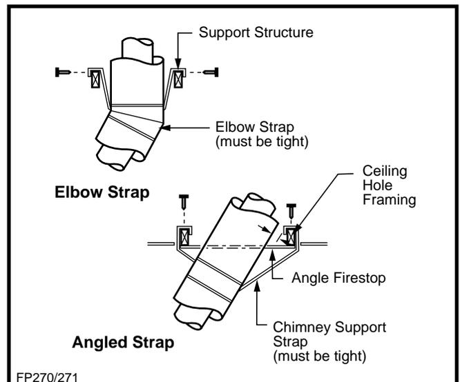
Fig. 15 Attach straps to a structural framing member.
