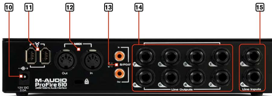
10. **Power Input ( - -⊕+ )** - Connect the 12VDC 2A power supply here when using ProFire 610 with a four-pin FireWire connection, or if your computer does not provide sufficient bus power on a 6-pin connection. If your computer can provide power over a 6-pin connection, it is not necessary to use the included power supply.
