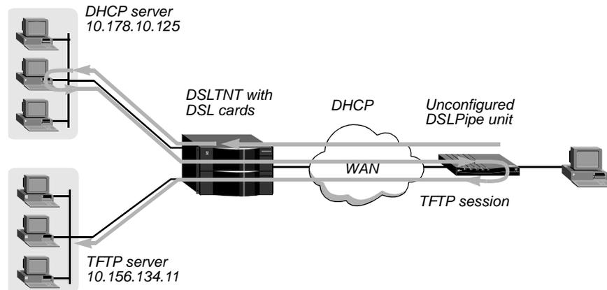
The DSLPipe unit uses the minimal configuration it obtains via DHCP to access the specified TFTP server and a configuration file, which is identified by a filename that matches the unit's serial number. After downloading the file, the DSLPipe begins using the configuration.
