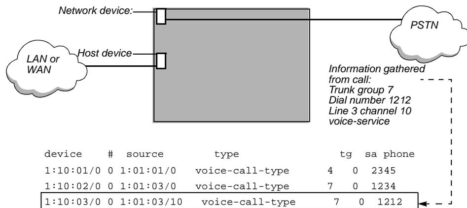
In the first entry, the preferred source is set to the first T1 line in slot 1, and the dial number is 2345. This entry passes the trunk group and subaddress comparisons, because both fields specify 0. It fails on the telephone number comparison and is dropped from the list.
