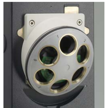
Fig. 11 Objective turret with labeled objective receptacles
