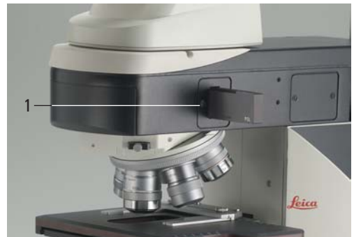
Fig. 29 Inserting the polarizer 1 The plug cap is replaced with the polarizer.
