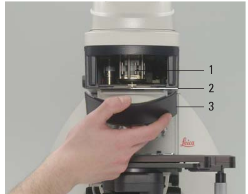
Fig. 26 Inserting the filter or reflector cubes
