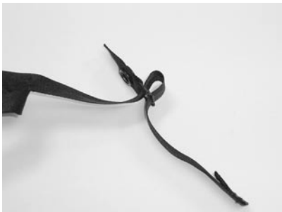
Figure 6-2 Lacing the Sliding Bar Buckle
