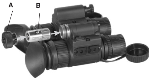
Figure 4-1 CR123A Battery Installation
