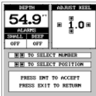
Note: Another way to use the keel offset feature is if you want to know the depth of the water below the lowest part of the boat, instead of the surface. To do this, measure the lowest part of the boat below the transducer. In this example, we'll use 3 feet. Now, using the keel offset feature, adjust the offset for a *negative* 3 feet.
