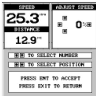
If the digital speed display is slower than your actual speed, add a positive percentage to make it read faster. If the digital speed display is faster, use a negative percentage to make it read slower. Use the arrow keys to change the speed, then press the ENT key. Press the EXIT key to erase this menu.
