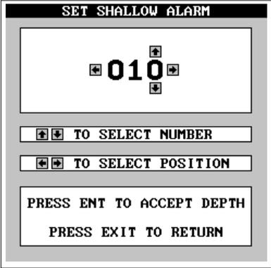
Press the ENT key to accept this setting. The unit returns to the alarms menu, showing a shallow depth of 10 feet. Now you can activate the alarm by highlighting the "Shallow Alm" label and pressing the right arrow key.
