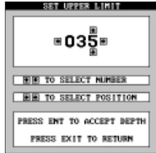
As you can see, the upper limit has changed from 0 to 35 feet. With the lower limit remaining at 60 feet, this gives a "zoom" of 25 feet. If you want to change the lower limit, repeat the above steps, press the right arrow key on the "Set Chart Limits" menu, and change the lower limit to the desired value.
