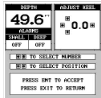
Press the right arrow key, then the up or down arrow keys until 1.0 appears in the "Adj Keel" box, as shown at right, then press the ENT key. This immediately changes the digital depth display at the top of the screen by one foot. Press the EXIT key to erase this menu.
