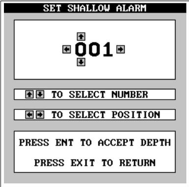
Use the up or down arrow keys to select the number, the right and left keys to move from number to number in the depth. For example, to set the shallow alarm depth to 10 feet, press the right arrow key once, then press the up arrow key once. The changes the second "0" to a "1". Next, press the right arrow key again and press the down arrow key once. This changes the "1" at the end of the number to a "0". The depth now shows 10 feet.
