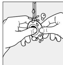
Remove the foam covers from the Speaker and Microphone and wash in mild soap and water.
