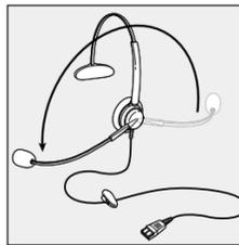
3. Rotate the Microphone Boom over the Headband to accommodate the left or right ear. Do not force the Boom beyond the built-in stops.
