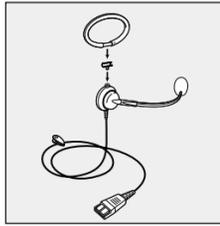
1. To attach the Earloop, detach the Earhook or Headband. Snap the T-Hinge onto the Earloop. Push the T-Hinge post into the post on the receiver.
