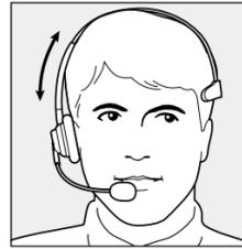
2. To wear the Headband, put the headset on with the speaker (receiver) covering your ear. Position the Stabilizer Cushion above your other ear. Adjust the length of the Headband.
