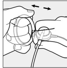
4. To remove the Earloop, position the Earloop away from the receiver and pull until it pops free.
