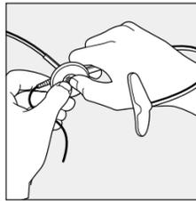
4. To remove the Headband, center both thumbs on the receiver foam and gently push outward until the Headband pops free.
