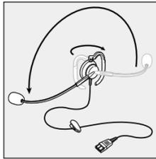
3. To wear on the opposite ear, rotate the Microphone Boom 180° and swing the Earhook to the opposite side of the receiver (speaker).
