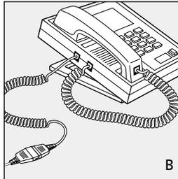
3. **A.** Connect the Quick Disconnect on the headset to the Quick Disconnect on the amplifier (follow the instructions included with the amplifier to connect it to the telephone system). To put a call on hold, unplug the Quick Disconnect.
