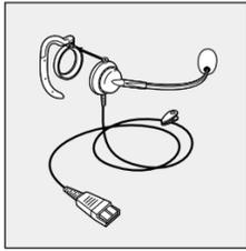
1. To attach the Earhook, remove the Earloop or Headband. Align the notch on the Earhook ring with the post on the receiver (speaker) and snap into place.
