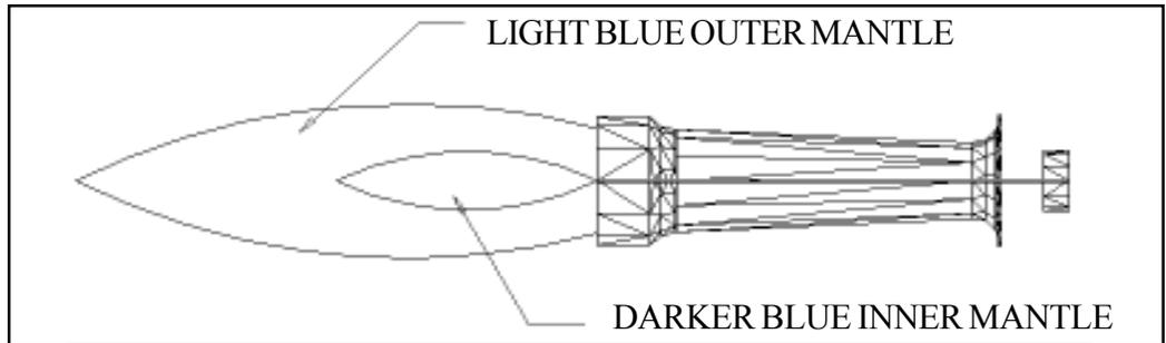
There is no primary air adjustment on the burner and with correct installation, a proper flame is assured; since the correct manifold pressure and orificing has been done at the factory for elevations up to 2,000 ft.
