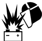
**GASES FROM BATTERY can explode.**
