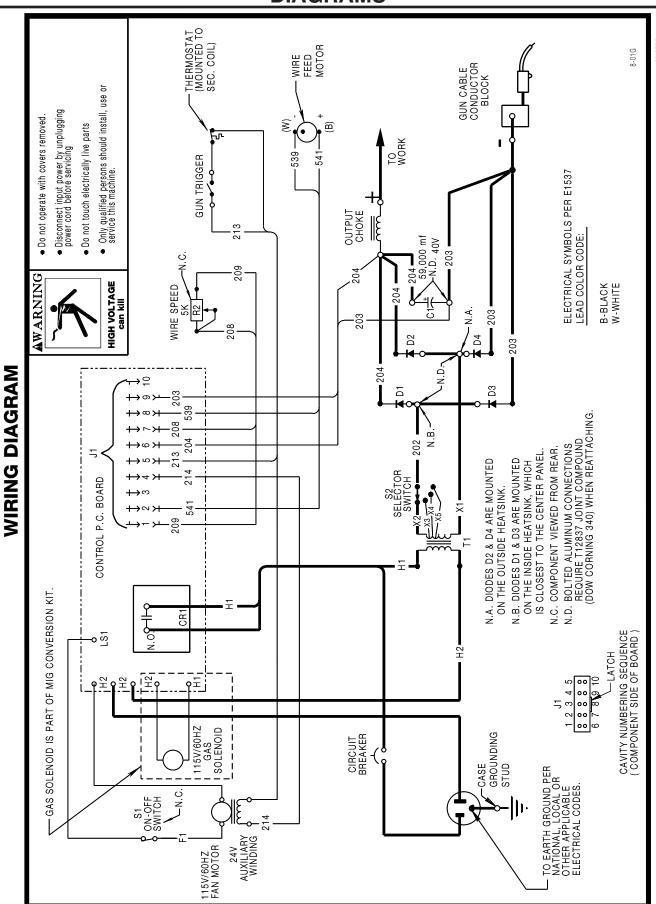
NOTE: This diagram is for reference only. It may not be accurate for all machines covered by this manual. The specific diagram for a particular code is pasted inside the machine on one of the enclosure panels.
