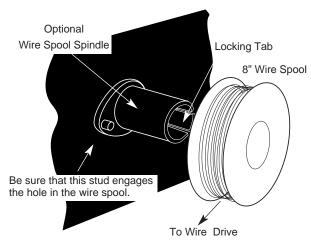
Wire Spool must be pushed all the way on the spindle so that the spindle's tab will hold it in place. The Wire Spool will rotate clockwise when wire is dereeled.
